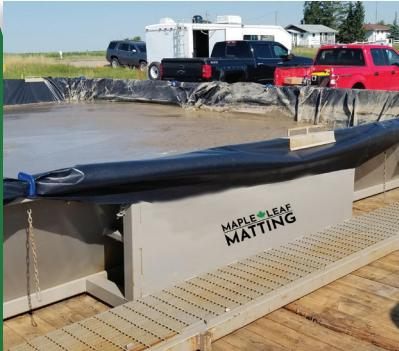
Maple Leaf Matting's **Slurry Cell containment system** offers our clients the unique opportunity to hold onsite slurry tailings from hydrovacs. Instead of housing multiple hydrovacs on location, our Slurry Cell system allows you to reduce costs by eliminating the requirement for multiple hydrovacs onsite, and travel to dispose of slurry tailings.
